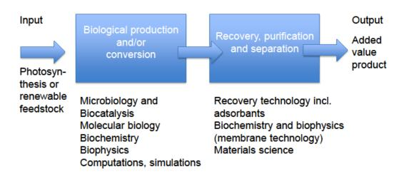
In the figure above the output arrow signifies high value products, e.g., fine and/or specialty chemicals, biologically-based materials or food and feed ingredients of high commercial value. The downstream box represents the technologies and processes needed to generate the high value output, e.g., purification and separation of compounds.
