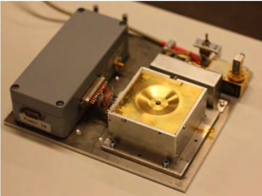
220GHz low-noise heterodyne receiver / transmitter with integrated antennas
